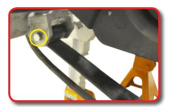
Use the jack to lower the rear end. Reposition spring above the axle and remount to factory mounting points using retained hardware from Steps 20 and 21.
