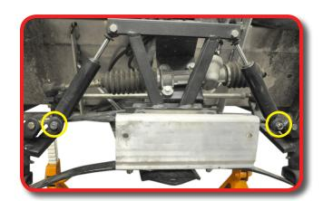
Remove A-Arm bolt from factory spindle on both sides. Do not retain bolts.
