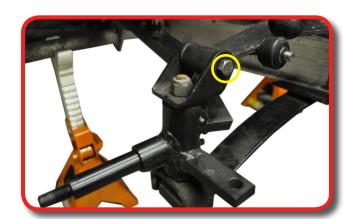
Remove the four factory A-arm bolts and nuts. Remove the factory A-arms, do not retain.
