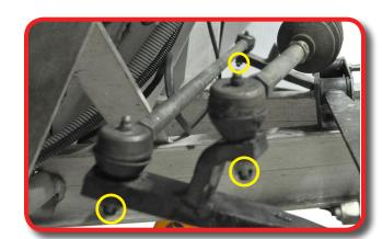
Remove the four bolts to detach factory suspension assembly and retain hardware. Factory suspension assembly will not be used.
