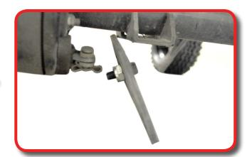
Place the rear shock mounting plate on top of leaf spring. Insert the lift block between the leaf spring and axle and then insert the provided U-bolt through top of the rear shock mounting plate. Attach shock to rear shock mounting plate.
