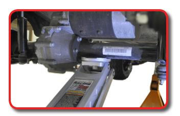
On drivers side completely remove nut from shock and factory U-bolts. Retain shock bushings and nut only.
