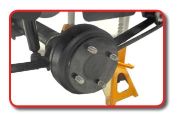
On passenger side loosen the factory shock and U-bolt. Do not completely remove the factory U-bolt, only loosen.
