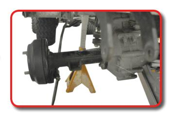
Attach bolt from hardware pack through the factory lower bracket. This bolt does not serve as a fastener, its only purpose to provide the proper placement of the bracket in the axle. Tighten all hardware.
