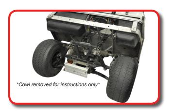
Using 19mm socket, remove front wheels.
