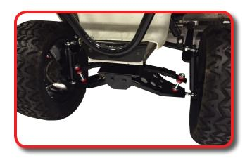
Chock front wheels. Lift up the rear of the cart using a jack. Use jack stands on the frame of the cart on each side to hold it up. Remove rear wheels using 19mm socket.
