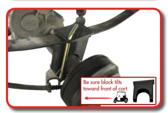
Attach factory lower bracket to U-bolts being sure that the bolt from step 23 fits properly into the hole in the axle. Tighten U-Bolts evenly.
