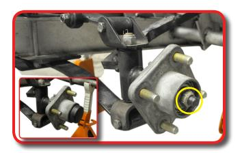
Remove lower shock mounting bolt and nut on driver and passenger side. Shock does not need to be completely removed, only the lower bolt so the shock can be pushed up and out of the way.
